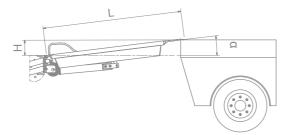
(H) of 100 mm using an electric pallet truck. By applying the formula indicated above, we obtain: LENGTH OF BRIDGE OR TAIL LIFT IN 4% for manual pallet trucks, 8% for walk-behind electric pallet MILLIMETRES (L) = 100 mm x 100 / 8 = 1250 mm You must therefore select a bridge or tail lift with a minimum length of 1250 mm.
